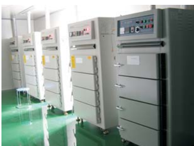
5. Bake and curing after encapsulation
