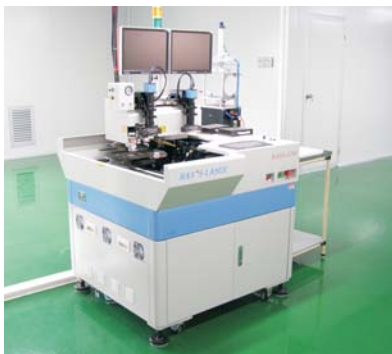
1. LED die separation + pick and place positioning on the Ceramic PCB
