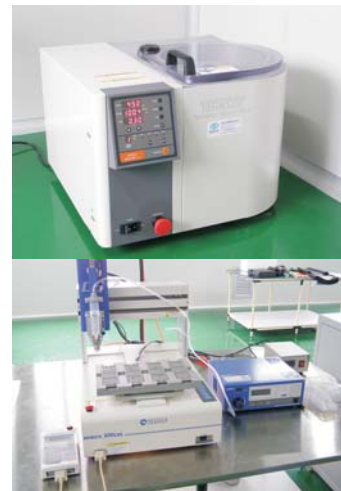
4. Phosphor deposition, encapsulation
